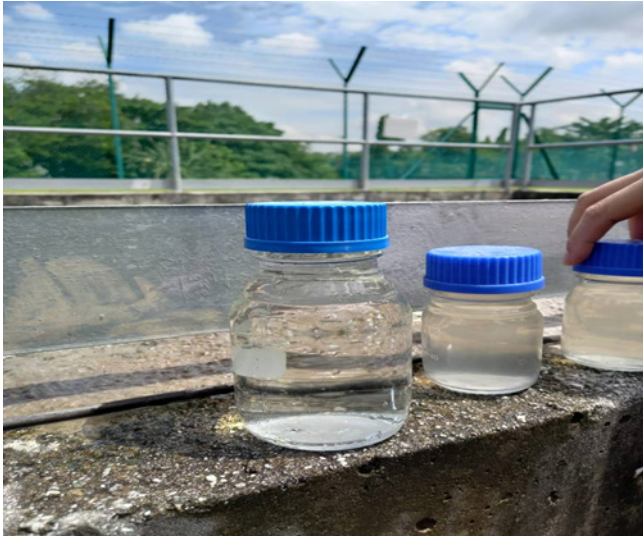
Fig. 4. The Comparison Between Treated Effluent (left) and Influent (right) (left diagram)
