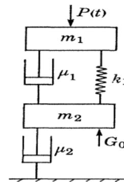
Figure 1. Pantograph Model (Ockendon and Tayler, 1971)
