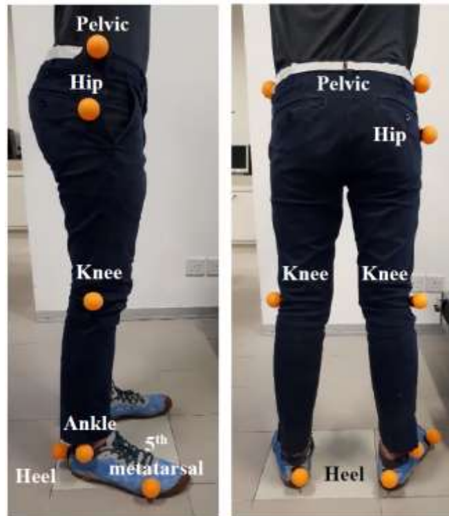
Figure 2. Markers placement on the sagittal plane (left) and back view of frontal plane (right)
