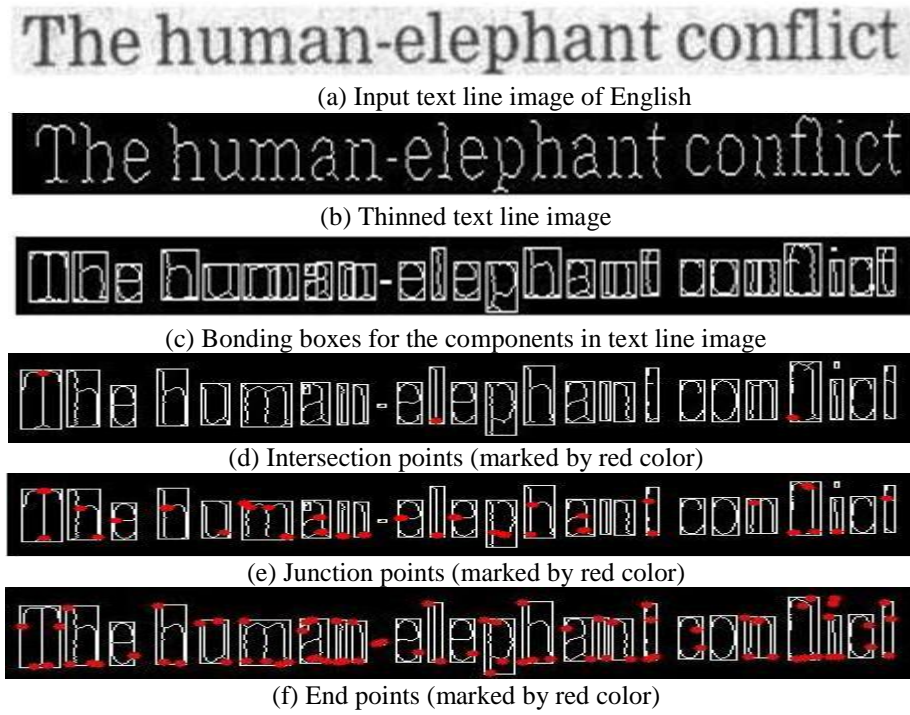
Fig. 4: Intermediate steps for the dominant pixel extraction
