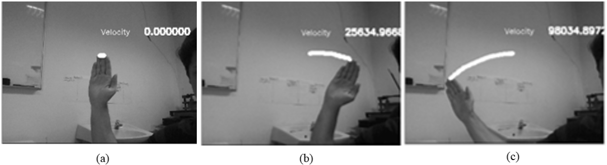
Fig 17: Velocity evaluation. (a) No motion; (b) slow motion; (c) fast motion.
