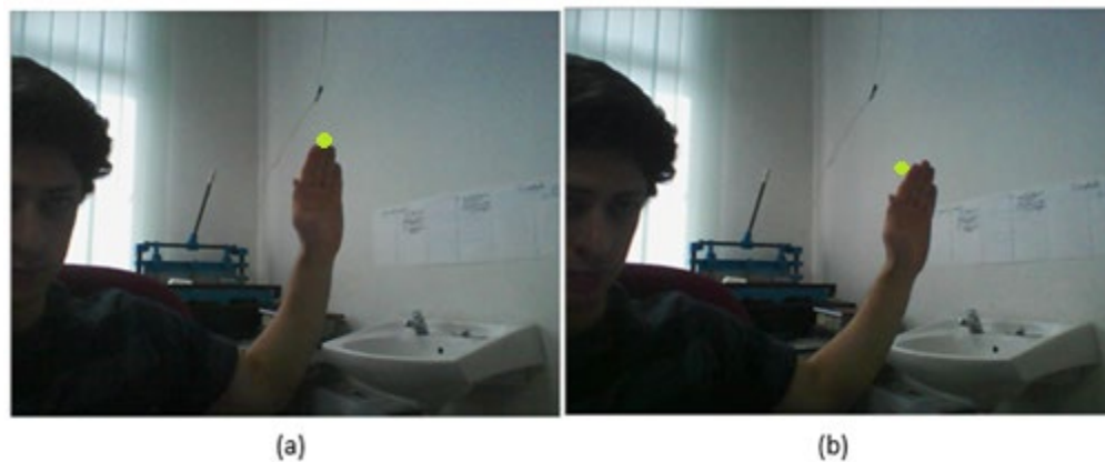
Fig 1: Kalman filter tracking. (a) Initial position; (b) Failure in tracking.
