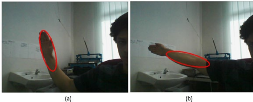
Fig 3: Cam-shift tracking (a) Initial position; (b) Failure in tracking.
