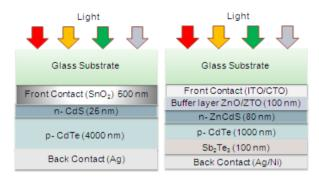
Fig. 1 Structures of the CdTe solar cells:
